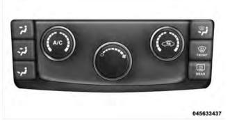
The Dual-Zone Manual Climate Controls allow both driver and front passenger seat occupants to select individual comfort settings. The controls consist of a series of outer rotary dials and inner push knobs.
